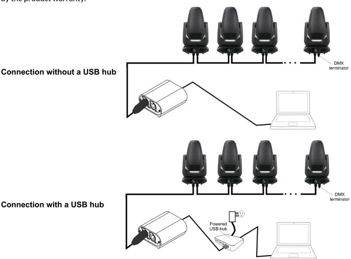
You can configure the NX DMX from the host PC once the system is installed.
